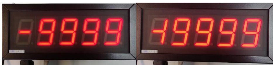
Fig. 75: Left — minimum in FULL DIGIT (-9999); right — HALF DIGIT (-19999).
